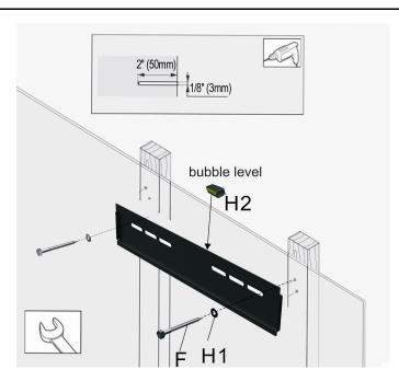
**CAUTION:** Do not over-tighten bolts - doing so may cause unnecessary damage to the wall. **CAUTION:** Do not release the wall plate until it is properly mounted and secured to the wall.
