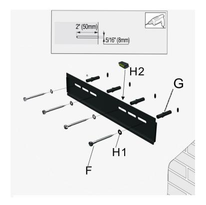
**CAUTION:** Do not over-tighten bolts - doing so may cause unnecessary damage to the wall. **CAUTION:** Do not release the wall plate until it is properly mounted and secured to the wall.
