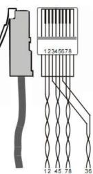
Notice: Cable connectors MUST be metal one, the shielded layer of cable MUST be connected to the connector's metal shell. to make a better transmission.
