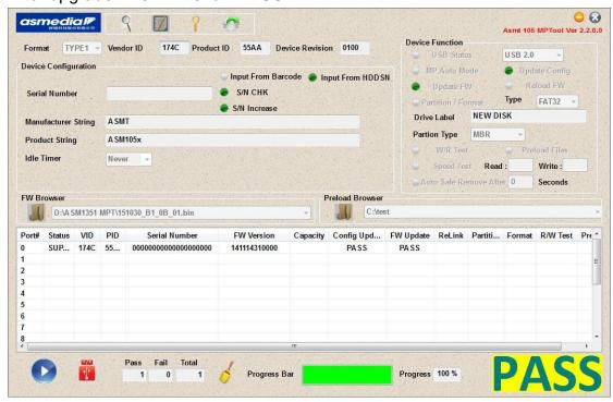
8. Safe to remove enclosure then reinsert, can see the FW Version is 151030b10b01
