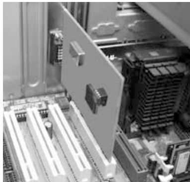
Figure 3. Inserting the PCI Board
