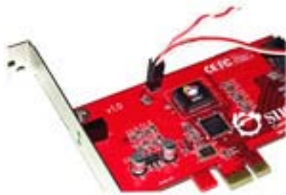
Figure 4. Connecting HDD LED
