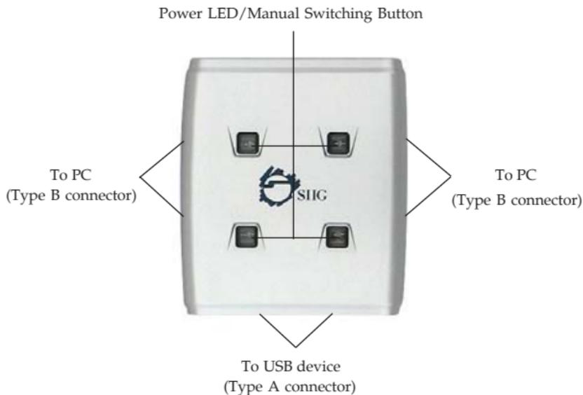
**Figure 2. USB 2.0 Switch 4-to-2 Layout**
