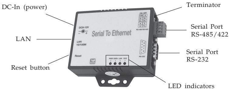
Figure 1: Serial Device Server
