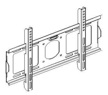
Fixed LCD / TFT TV Wall Mount Material: 2.0mm Cold Rolled Steel Plate TV Size: 32" - 60" Max load capacity:165 lbs / 75 kgs Wall distance: 30mm / 1.2" Bubble level system included Universal Mounting Pattern
