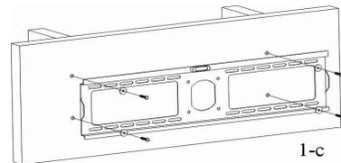
**CAUTION:** Do not over-tighten bolts-doing so many cause unnecessary damage to the wall. Avoid excessive torque.
