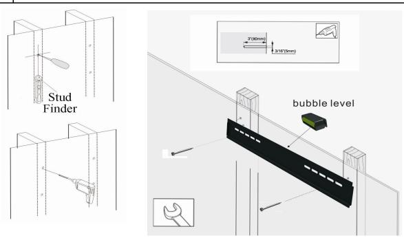
**CAUTION:** Do not over-tighten bolts - doing so may cause unnecessary damage to the wall. **CAUTION:** Do not release the wall plate until it is properly mounted and secured to the wall.
