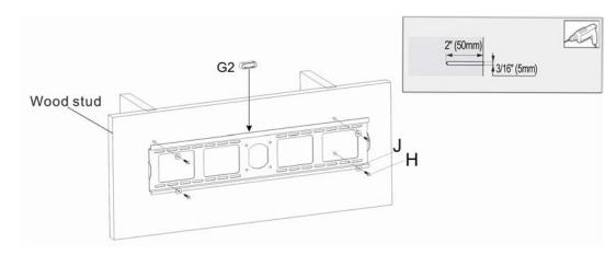
CAUTION: Do not over-tighten bolts-doing so many cause unnecessary damage to the wall. Avoid excessive
