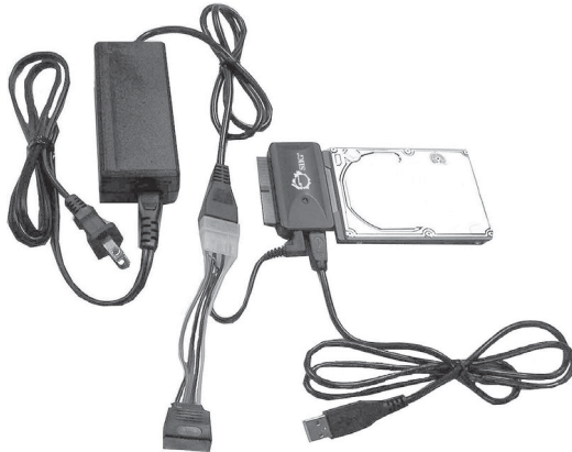
Figure 2: Connecting 2.5" IDE HDD
