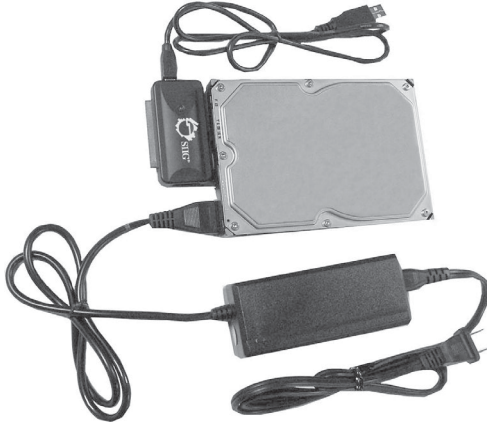
Figure 3: Connecting 3.5 IDE HDD
