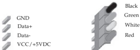
Figure 2: USB Pin-out Header
