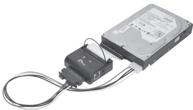
Figure 3: Connecting 3.5" IDE HDD
