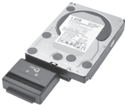
Figure 4: Connecting SATA HDD
