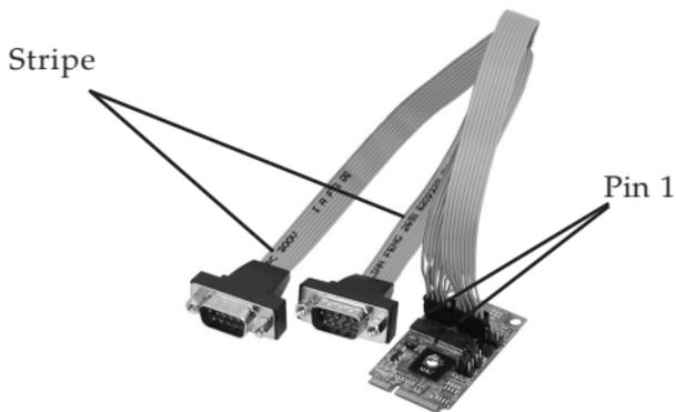
Figure 4: DB9 Flat Cable Connection
