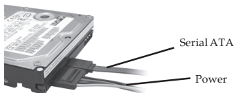
Figure 2. SATA hard disk drive connections
