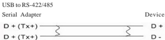
The adapter comes with Tx and Rx termination resistors for each serial port. You can configure the jumper settings to avoid impedance mismatched problems.
