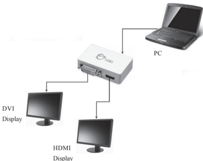
One PC can connect up to three *USB 3.0 to HDMI/DVI Dual Display Adapters*, equivalent to up to six monitors.
