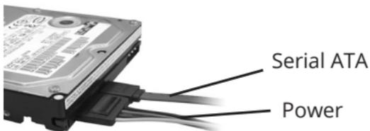
**Figure 3: SATA hard disk drive connections**
