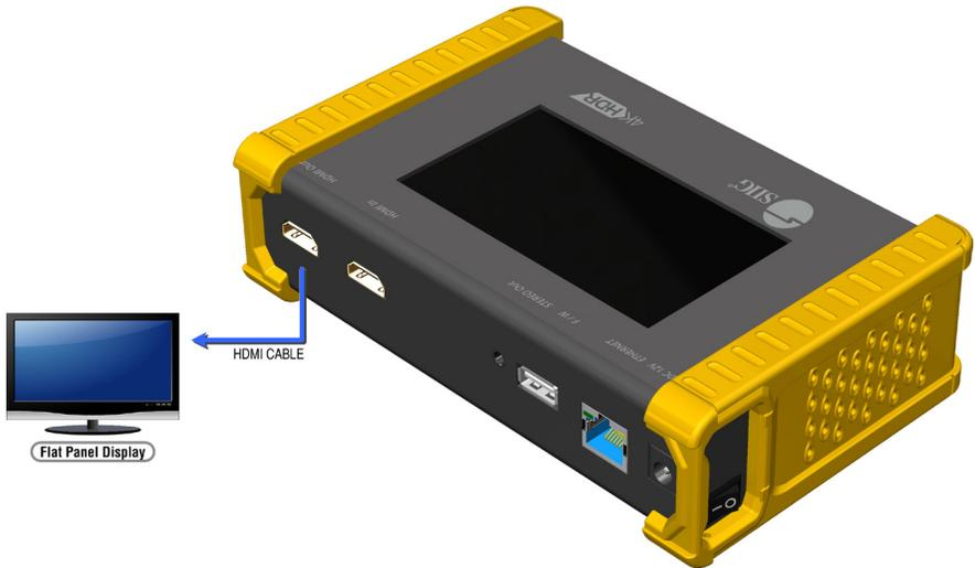
After making the physical connections between Generator and the display device. User can select different generator function to display on the sink device under test.
