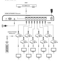
Cascaded with LAN Switch can use more than 8 ports
