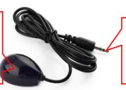
3.5mm jack, insert it into the IR receiver socket to connect the IR with the amplifier
