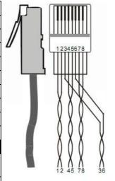
Notice: Cable connectors MUST be metal one, the shielded layer of cable MUST be connected to the connector's metal shell, to make a better transmission.
