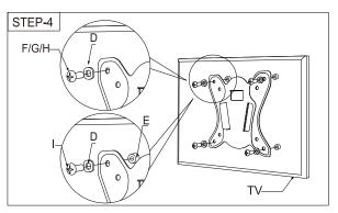
Step4: Select the right screw sets from the screw packing and install the TV Plate onto the back of the TV.
