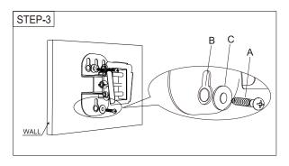
Step3: Fix the wall dead plate with three lag bolts to install the wall fixed installation for the panel TV on the vertical wall.
