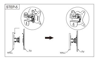
Step5: Hang the TV Plate with the TV Set onto the arm connect part and screw tighten at last.
