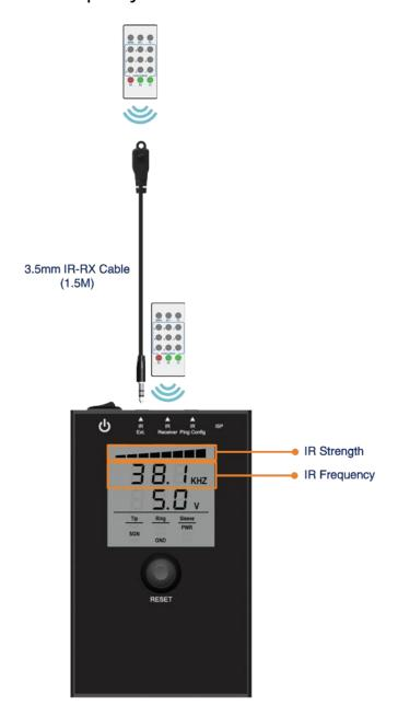
2) Measure IR Jack Power Voltage & Pin Configuration
