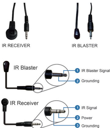
Figure 5: IR Cable Pin Definition
